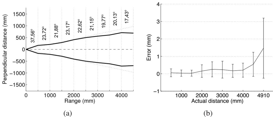
The errors between the actual and the measured ranges have been computed. The mean and the standard deviation of these errors are shown in Figure 3b. It can be observed how the mean and the standard deviation of the errors tend to increase with distance.
