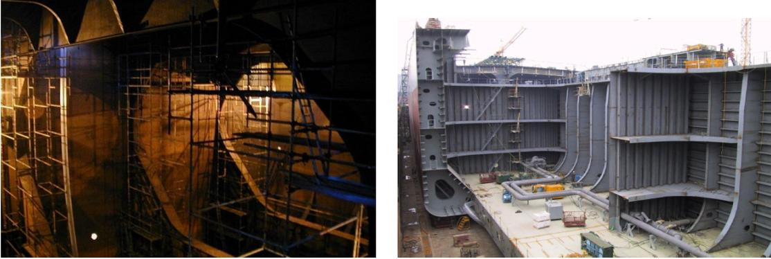
Figure 1: (left) Staging required during a vessel inspection. (right) Oil tanker in shipyard during construction.
