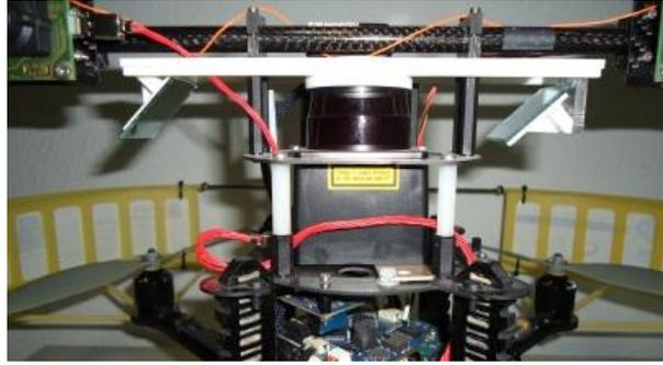
Fig. 3: Laser-based altimeter (left), as well as distance to ceiling estimator (right), by deflecting selected laser beams using mirrors.
