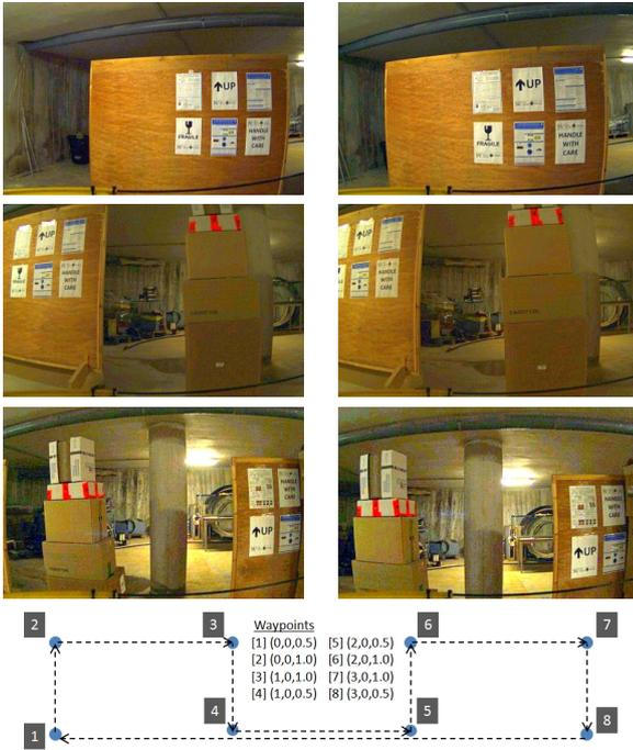
Fig. 10. Pairs of images taken at the same location in two different executions of the last experiment. The slight deviations in viewpoint are due to the orientation accuracy parameter, set to 6 degrees in the mission specification file. The drawing at the bottom shows the positions where the photos are to be taken during the inspection mission. The pairs above correspond to, respectively, locations 2, 4 and 6.
