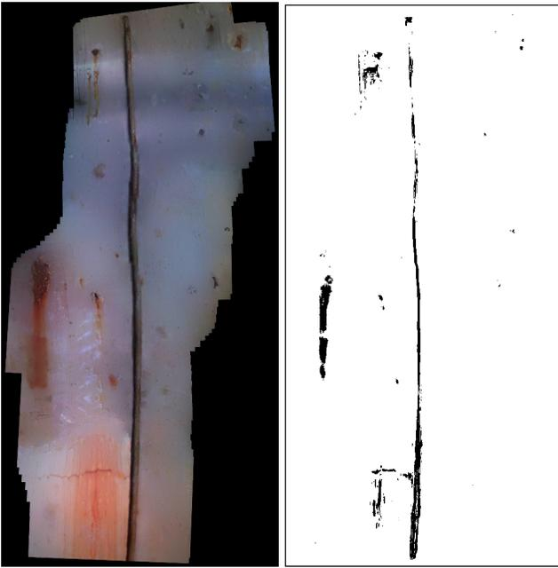
Fig. 8. (left) Mosaic using the images collected by the MAV in a top-down trajectory [mosaic contrast has been tuned for visualization purposes]. (right) Defective areas found, shown in black.
