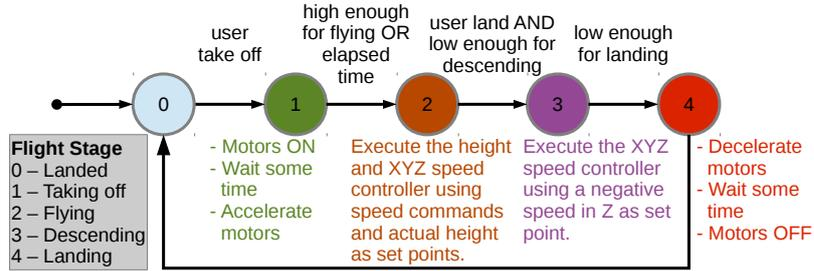
Fig. 4. Flight control state machine.
