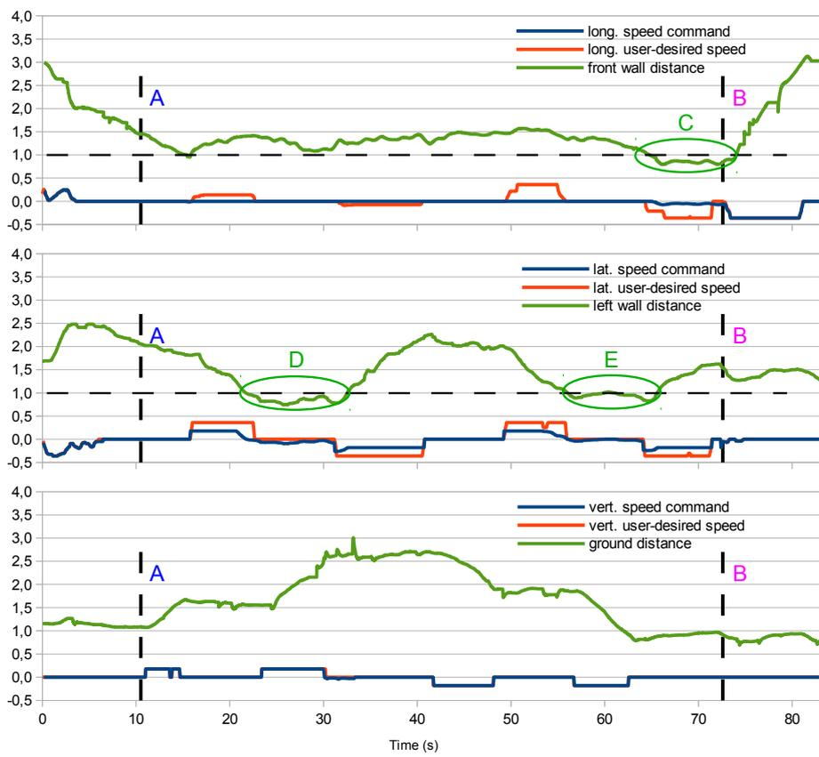
Fig. 13. Performance of the platform during an inspection task using the inspection mode (A→B). All units are in SI (m or m/s accordingly).
