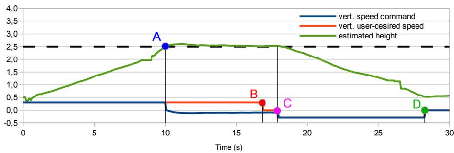
Fig. 8. Performance of the *limit\_max\_height* behavior: the user-desired vertical speed is obeyed until the platform reaches the maximum allowed height (→A), then the desired vertical speed is ignored (A→B) until it becomes zero (B→C), and finally the platform descends following again the desired speed (C→D). All units are in SI (m or m/s accordingly).
