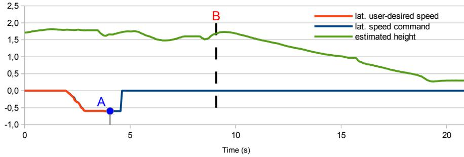
Fig. 9. Performance of the *waiting\_for\_connectivity* behavior: the communication with the base station is lost during the flight ( $\rightarrow$ A), what makes the behavior force a hovering maneuver (A $\rightarrow$ B) while the vehicle tries to reconnect; after waiting for five seconds without success, the behavior makes the platform land (B $\rightarrow$ ). All units are in SI (m or m/s accordingly).
