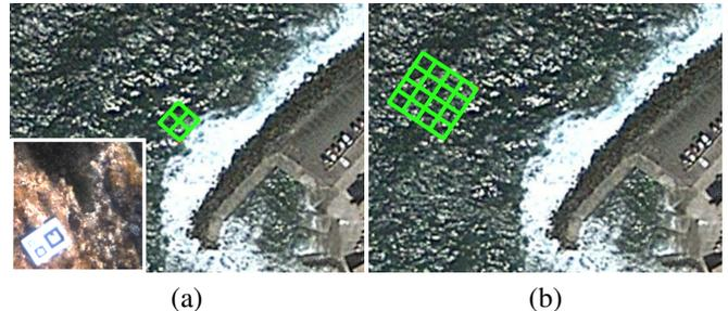
FIG. 7: Two programmed missions on the AUV control application which integrates Google Maps. (a) Small mission of  $10m \times 12m$  with an *AR-Marker* installed on the seabed at a specific point and (b) large mission of  $20m \times 22m$ .
