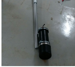
(A) USBL fixation to buoy pole.
