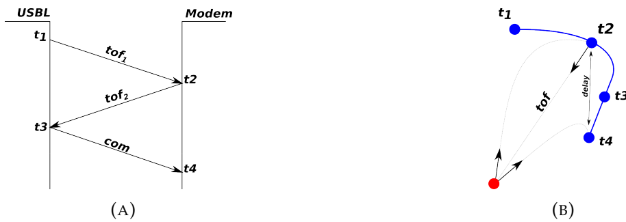
FIGURE 3.5: USBL measurement TOF and delay. Where t_{measurement} = t_2 is the time in which the modem listens the query and answers
