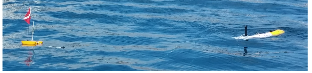
(B) AUV with the catamaran shaped WLAN link tethered.
