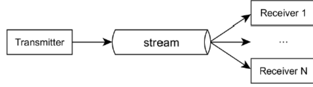
Figure 2.2: Stream-based communication scheme (reprinted as it appears in [6] Fig. 5)
