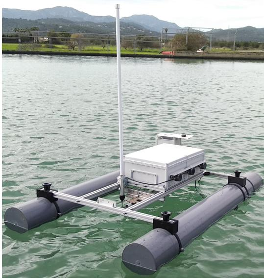
Figure 5. Xiroi ASV at the outdoor pond where the experiments were performed.
