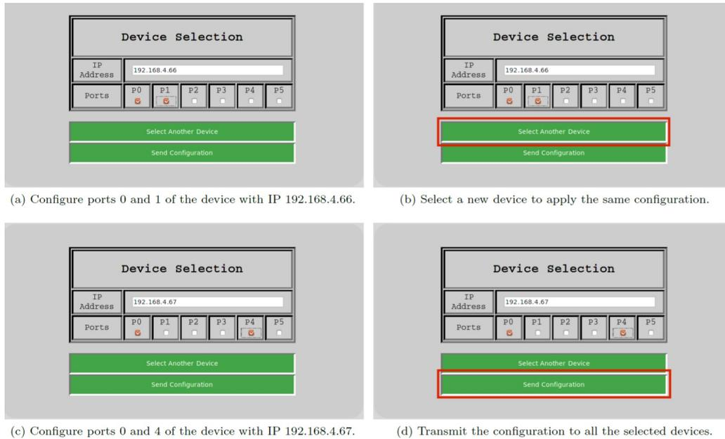
Figure 4.7: Steps in Device Selection Menu to set the configuration in the desired ports.
