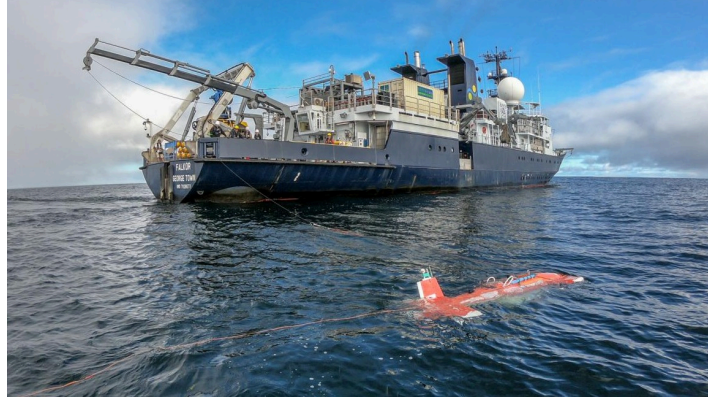
Figure 5.11: AE2000f AUV being deployed in Hydrate Ridge in front of R/V Falkor.
