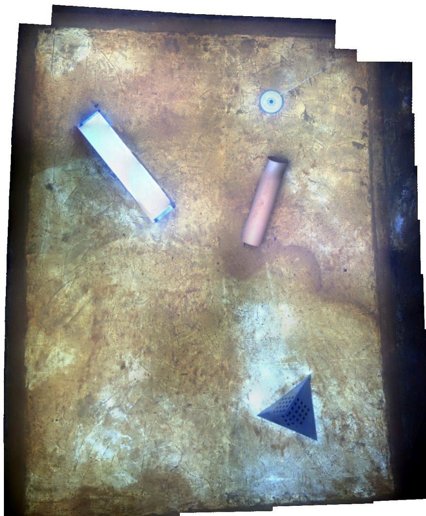
Figure 4.12: Pool mosaic built from a subset of 40 images (left camera of stereo dataset). From [7].
